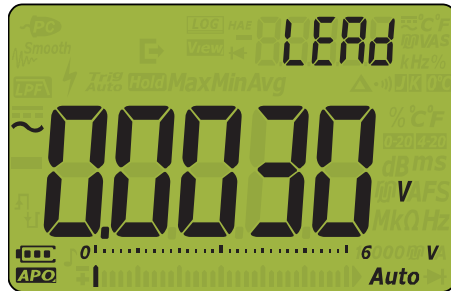
Figure 1-5 Input warning display
