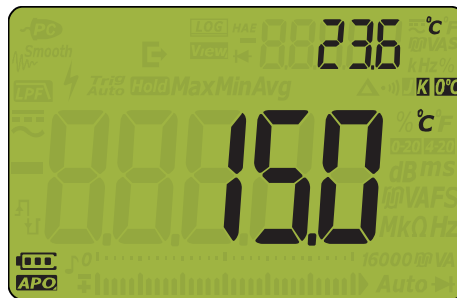
Figure 2-25 Temperature measurement without ambient compensation
