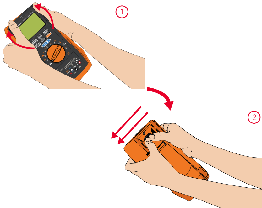
Figure 1-1 Removing the orange rubber holster
