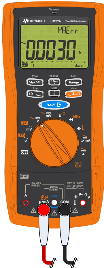
Figure 1-4 Example of wrong terminal input
