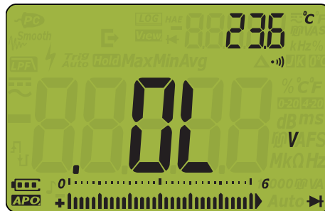
Figure 2-17 Open diode display
