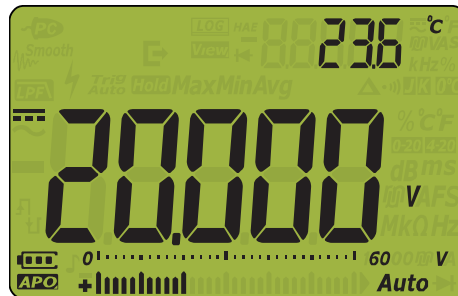
Figure 2-6 DC voltage display
