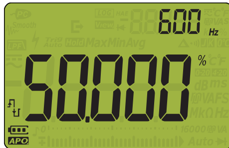
Figure 2-35 Square wave output display
