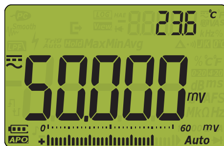
Figure 2-8 AC+DC voltage display
