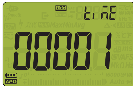
Figure 4-6 tiME display - data logging
