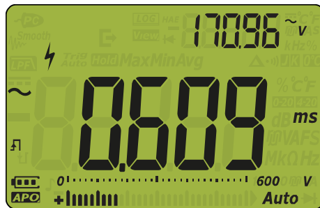
Figure 2-33 Pulse width display
