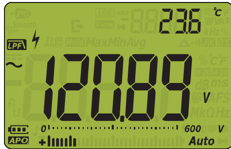
Figure 2-5 AC voltage (with LPF) display
