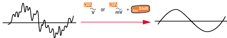
Figure 2-4 Low-pass filter operation
