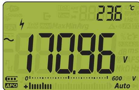
Figure 2-1 AC voltage display
