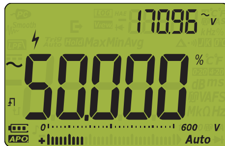
Figure 2-34 Duty cycle display
